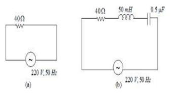
The rms current in circuit (b) can be larger <sup>a)</sup> than that in (a)
